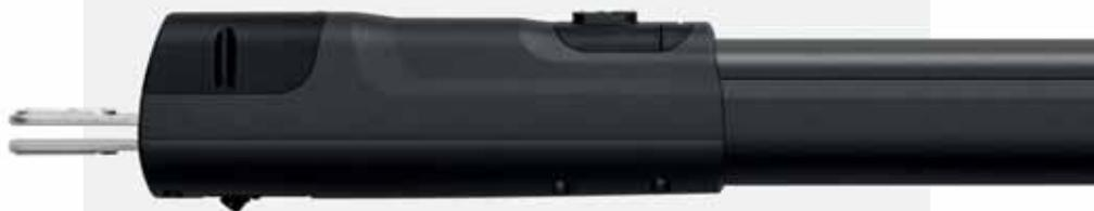
Reliable and innovative irreversible telescopic gear motor, available in 230 Vac or 24 Vdc, characterised by 2 mechanical stops in opening and closing accessible from above and easy to adjust. With its compact dimensions (only 96 mm wide), TOM is designed with the highest quality materials: bronze alloy release wheel, worm protected by a scraper ring and stainless steel stem, suitable for use in dusty and sandy environments or where there are aggressive atmospheric agents.
