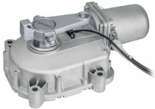
Irreversible electromechanical geared motor available in 230 Vac and 24 Vdc version, with the option of opening to 180°. Full metal mechanics and built-in mechanical stop. It's available a model equipped with 10 m cable to facilitate wiring and prevent problems linked to the oxidation of electrical contacts (DU.IT14N-10/DU.IT14NVE-10).
